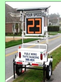
The portable speed trailer visually displays drivers' real-time speed; therefore, it may be effective in increasing awareness of local speed limits.
